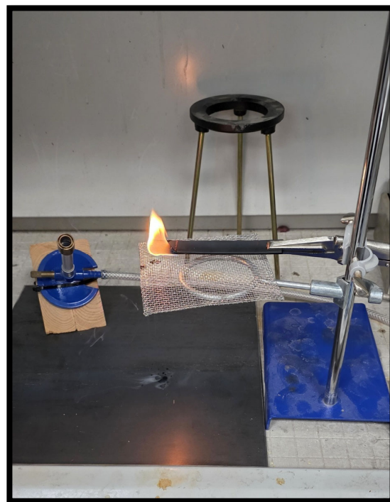
ASTM D635, Rate of Burn Test
