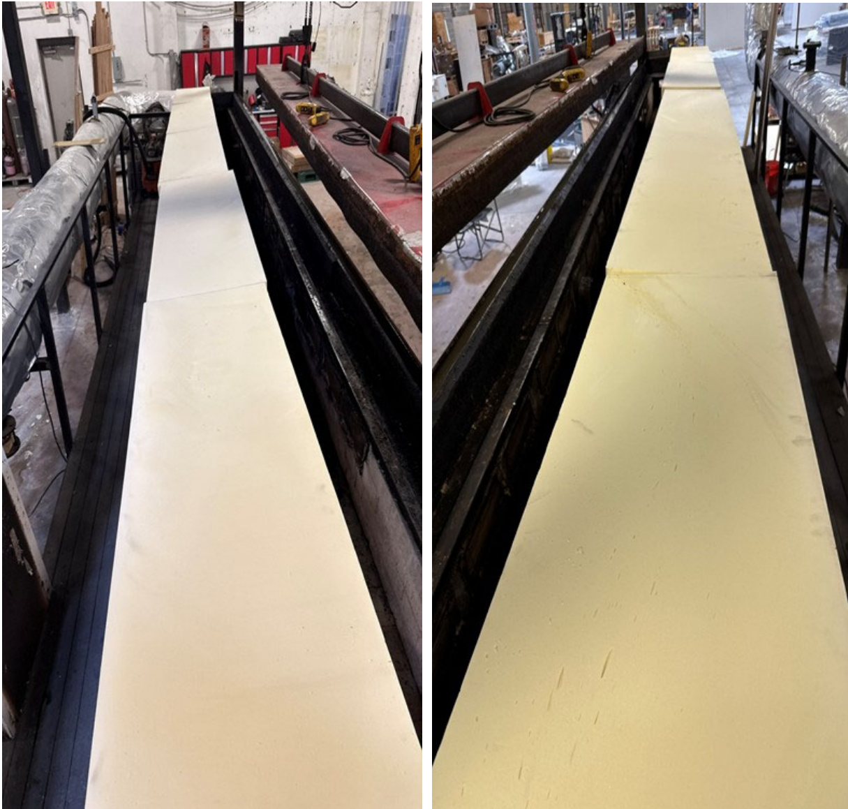
Photograph No. 1: Test specimen prior to testing showing the entire 24-foot test specimen from the fire exposure chamber's burner end (left), and vent end (right).
