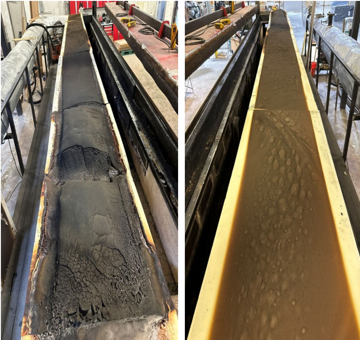
Photograph No. 2: Test specimen from the test chambers burner end (left), and vent end (right) showing the post 10-minute test sample condition immediately after removal from the test chamber.
